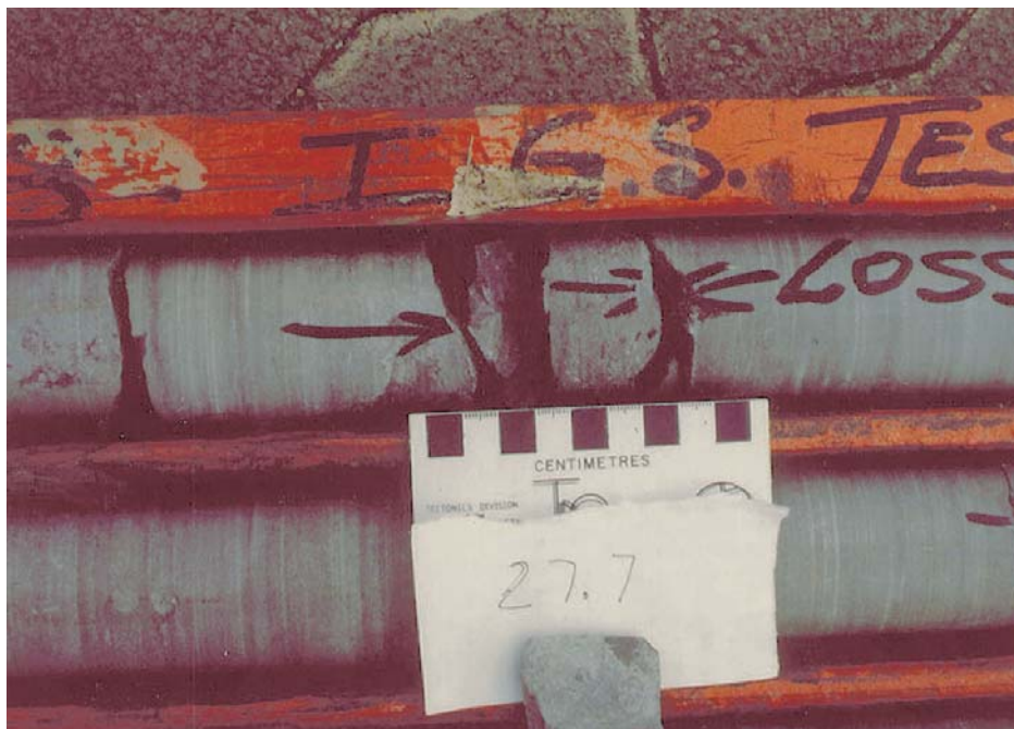
Figure 5–26 Detailed view of the fracture in Figure 5–24. Substantial water loss was incurred along this 80 mm fracture zone during the drilling.
