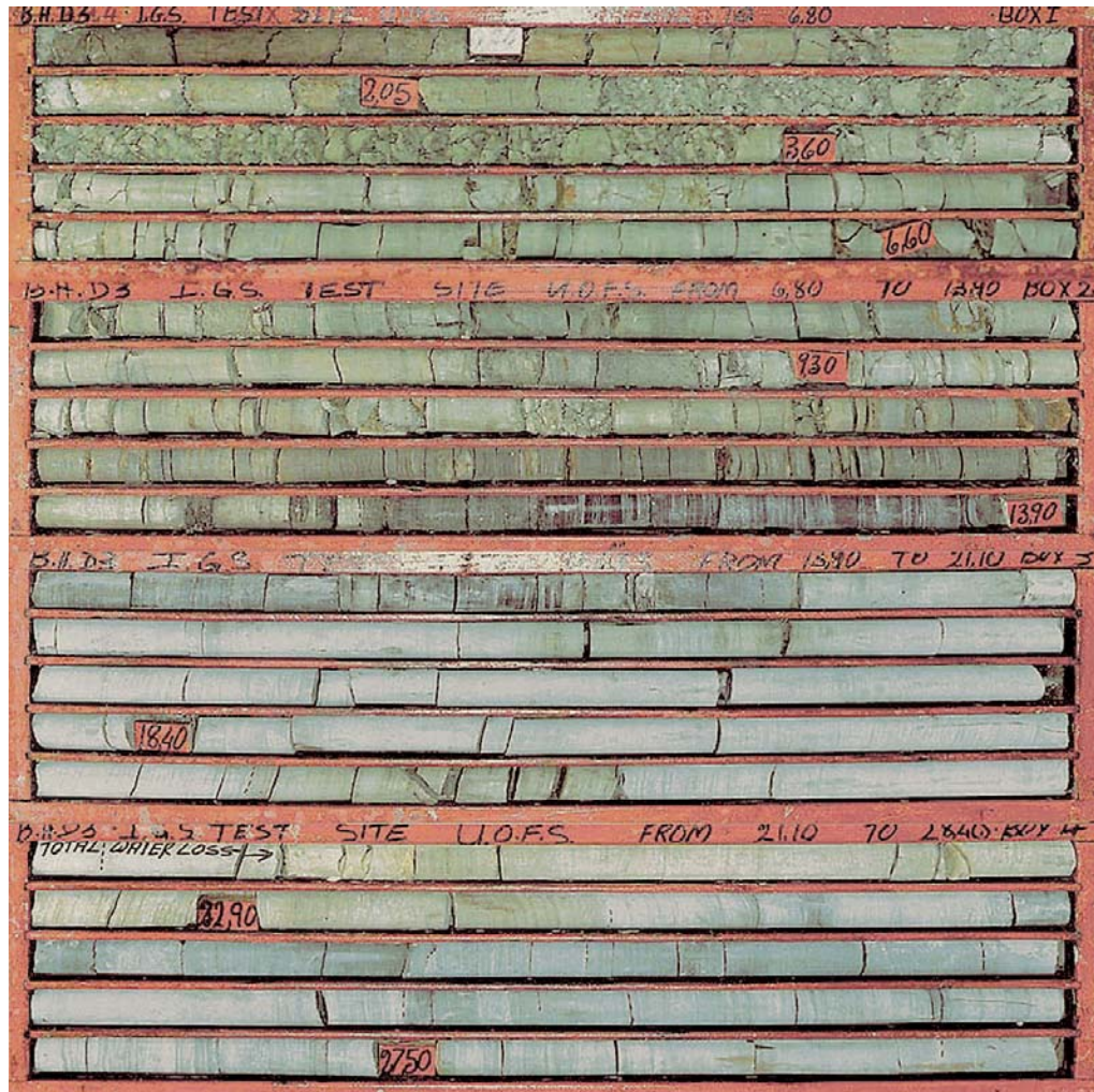
Figure 5–24 Photograph of a part of the core from Borehole CH3. Notice in particular the fracture marked with the comment ‘total water loss’.
