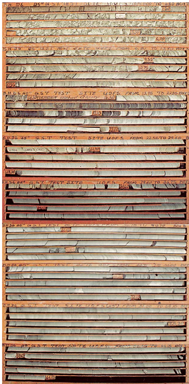
Figure 4-9 Photograph of cores from borehole CH6 on the Campus Test Site. The borehole is inclined at an angle of 45°.
