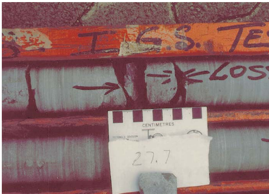
Figure 1 Photograph of the water-yielding fracture in a core sample from the Campus Test Site.
